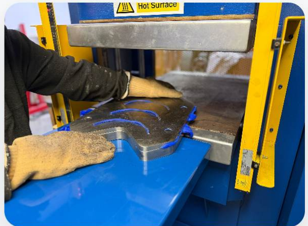
Loading a mould tool into one of our compression presses in Worthing
